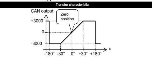
Default 0°: horizontal (label upwards), no acceleration applied. To eliminate mounting offsets the sensor can be centered within ±5° tilt (by the CAN object dictionary)
