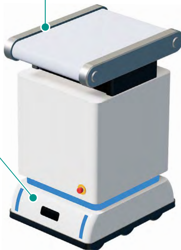
Application: Autonomous transportation robot with belt conveyor
