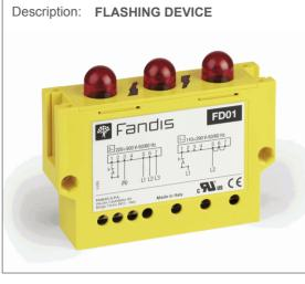
Casing material: Protection degree: Fixing system: Electrical connection: Electrical section wires: Rated insulation voltage: Storage temperature: Dimensions: Weight: Approvals: plastic IP20, according to IEC 529/ EN 60529 by two screws M4 by screw terminals from 0,5mm² to 2,5mm² 500 V from -30°C to +80°C 30x110x86 mm 0,100 Kg CE, cURus
