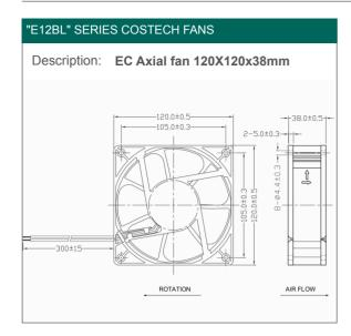
Casing material:Thermoplastic in black color, UL 94 V-0Impeller materialThermoplastic in black color, UL 94 V-0Protection degree:IP20, according to EN 60529 standardFixing system:by No 4 M4 screws
