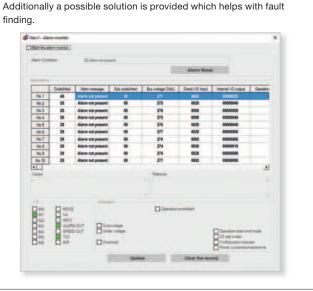
When an alarm occurs the details of the alarm are recorded as well
