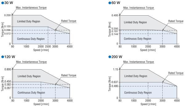
• The values correspond to each specification and characteristics of a stand-alone motor. The speed - torque characteristics show the values when rated voltage is applied.
